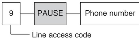
**Example-2:** If transmission errors occur when making an overseas transmission, add two pauses at the end of the phone number.
