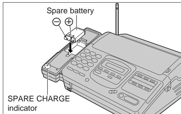
The spare battery is always being charged in the main unit while the power cord is connected. The battery cannot be overcharged.
