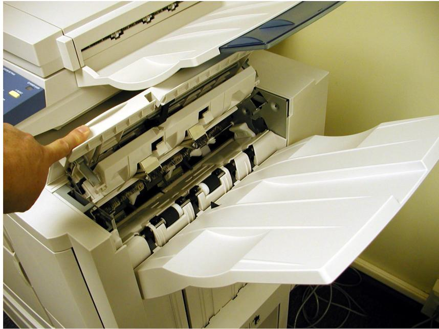
**Figure 16** – The finisher's misfeed-access area.
