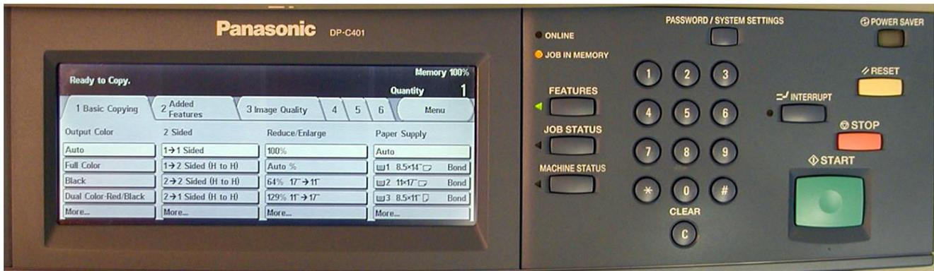
Figure 10 – The Panasonic WORKio DP-C401’s control panel.
