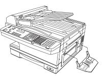
Attach the paper tray by inserting its two pegs at a slightly upward angle into the appropriate holes, as shown.
