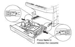
2 On the rear side of the cassette, you will see the pin and three sets of holes. Note the drawing below. If the pin is in the upper and lower set of holes, your fax "thinks" the cassette holds letter-sized paper. If the pin is in the middle and lower holes, your fax thinks the cassette has legal-sized paper.
