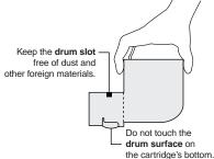
**8** Gently install the toner cartridge in the printer, making sure the toner cartridge's four pins fit in the slits inside the printer frame.
