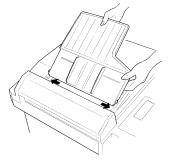
Attach the Multi paper tray by inserting its two pegs at a slightly upward angle into the appropriate holes, as shown.
