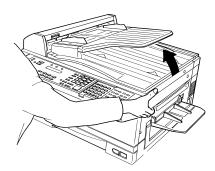
**2** Pull up the *printer cover release* and open the printer cover.
