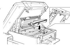
**9** Insert the fuser cleaner into the slot in the fuser unit. The fuser cleaner cleans the fuser unit roller.
