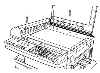
**2** Get the protection seals from your manual kit, and attach one protection seal on each transport screw's now-open hole. This shields the hole while you are using the machine.
