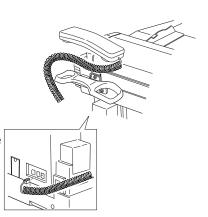
**5** Place the telephone handset onto the handset cradle. The cradle will press the handset's "flash" button, hanging up the handset.
