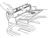
**3** Gently close the scanner cover, making sure both sides are snapped down securely.
