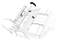
**7** Use the cloth with isopropyl alcohol to clean the contact glass.
