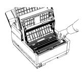
4 Remove the new toner cartridge from its package and gently shake it from side to side to distribute the toner.
