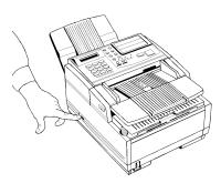
2 Plug the power cord into the back of the unit.
