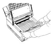
**3** Pull the blue lever on the old toner cartridge all the way toward you. Carefully pull the old toner cartridge out of the image drum unit. Dispose of it in the plastic bag you received with your new cartridge.
