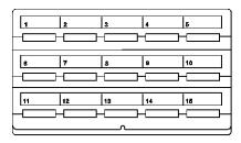
The One Touch keys are your fax machine's most important tool. Use them for quick, one-touch dialing, and to access most functions and programming options.
