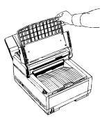
**2** Push in the cover release buttons on the side of the copy stacker until you hear a click. Lift the copy stacker.
