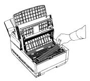
4 Push the lever forward to secure the cartridge.
