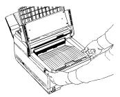
3 Remove the old image drum unit (with its toner cartridge), wrap it in the packaging materials from your new image drum unit, and discard it.
