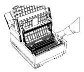
7 Using the cleaning wipe provided with your new toner cartridge, gently wipe back and forth across the full length of the LED array. Let the array dry completely.
