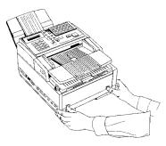
3 Pull the manual paper feeder down until it is horizontal.
