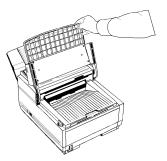
**2** Push the buttons on the side of the copy stacker until you hear a click. Lift the copy stacker up.
