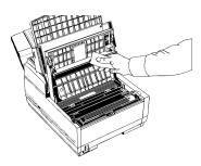
**8** Close the copy stacker and push down until you hear the copy stacker click into place. Be sure that the cover latches on both sides.
