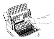
10 Close the copy stacker and push down until you hear the copy stacker click into place. Be sure that the cover latches on both sides.
