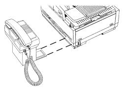
3 Plug one end of the handset cord into the handset and the other end into the jack on the front of the cradle. Place the handset in the cradle.
