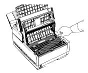
6 Once the toner cartridge is in place, push the lever all the way toward the back of the fax machine to secure it and release the toner.
