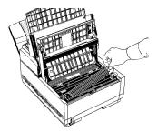
**8** Once the toner cartridge is in place, push the lever all the way toward the back of the fax machine to secure it and release the toner.
