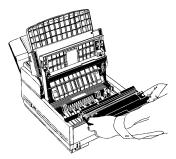
**4** Remove the protective sheet. Be careful not to touch the green surface of the drum.
