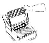
**2** Press in the cover release buttons on the side of the copy stacker until it clicks open. Lift up the stacker.
