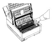
**9** Using the cleaning wipe provided with your new toner cartridge, gently wipe back and forth across the full length of the LED array. Let the array dry completely.
