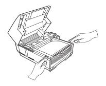
4 Grasp the image drum and lift it out of the machine. Set it aside on a clean, dry surface out of direct sunlight.
