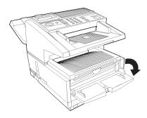
3 Insert a sheet of paper (face up) on the tray and push into the slot until the machine grabs hold of the paper.
