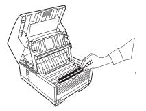
8 Push the lock lever (in the direction of the arrow) until it stops.
