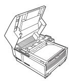
**3** Press the release buttons located on both sides of the copy stacker. Lift up the stacker.
