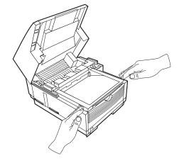
**3** Move aside the protective sheet and grasp the image drum cartridge, then lift it out.
