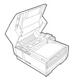
**3** Press on the latches on both sides of the copier stacker until the cover of the image drum compartment is released and pops up. Lift up and back, revealing the image drum.
