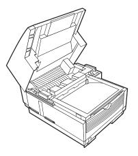
**2** Press the release buttons located on both sides of the copy stacker. Lift up the stacker.
