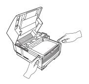
5 Insert the new drum cartridge. Press down firmly on both ends to lock the drum in place.
