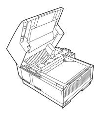
2 Press the release buttons located on both sides of the copy stacker. Lift up the stacker.
