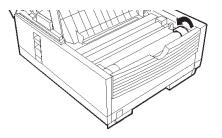
**9** Use the cleaning wipe provided with your new toner cartridge. Gently wipe back and forth across the full length of the LED array. Use a clean section of the wipe with each pass.
