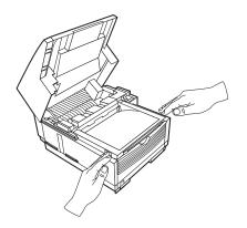
**3** Pull the lock lever on the toner cartridge in the direction of the arrow.
