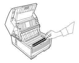
**5** Push the lock lever (in the direction of the arrow) until it stops.
