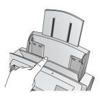
2 Fan, neatly stack, then insert up to 100 sheets of paper.
