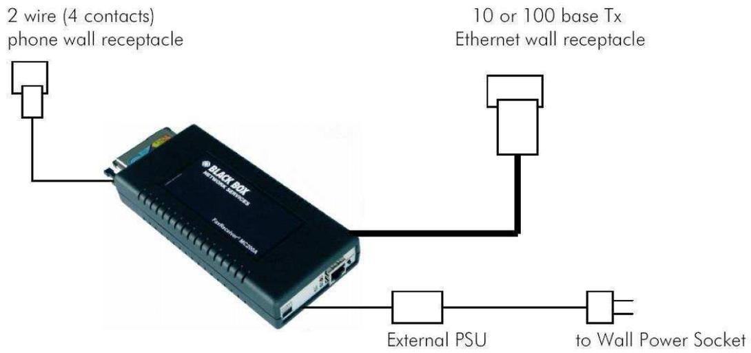
Installation where an outgoing fax machine is required on incoming line:
