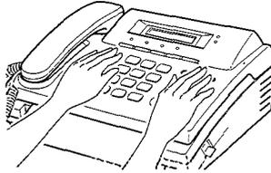
◀ Press down on the Cover using both hands until it snaps into place.
