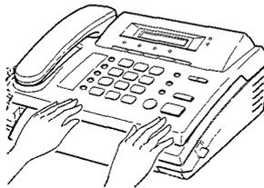
◀ Press down on the Cover using both hands until it snaps into place.
