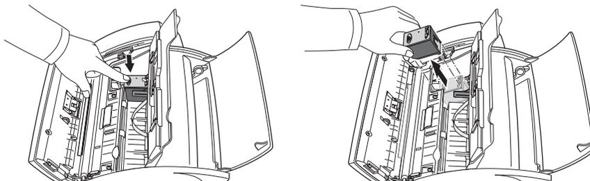
**5** To load the cartridge insert the cartridge below the metal clip and pointing down at the front. When the cartridge is pushed to the back of the cartridge carrier lift the front of the cartridge up until it clicks into place.
