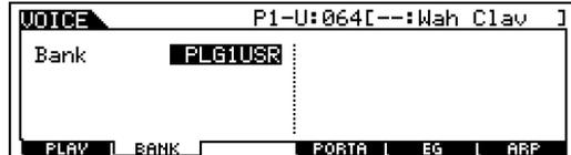
The PLG\_USR bank (PLG1USR in our example slot 1) will allow you to create and store 64 sounds based on the data on the PLG150-PF board. This Voice data will remain in memory after power down. And will be available as long as the PLG150-PF board has been detected and is in the slot.
