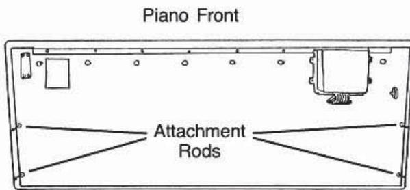
Pictured are the attachment rods on the piano bottom.
