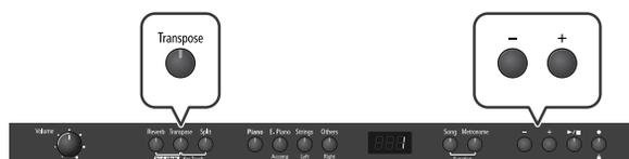
On the RP201, you can transpose the pitch of just the keyboard, or the pitch of the keyboard and song together, or the pitch of just the song (Playback Transpose; p. 29) (Transpose Mode; p. 35).
