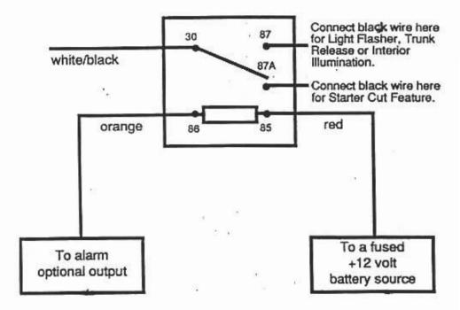
Wire the relay as shown in the alarm installation/operation guide.
