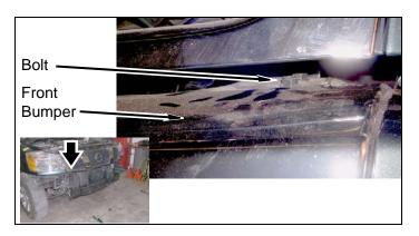
Install front bumper and two kit spacers on front bumper brackets with two kit bolts (M8-1.25 X 40mm). Do not tighten.
