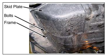
m. Mark and drill two 1/4" holes into skid plate. Install front bumper fascia straps onto skid plate with two kit **push clips**.
