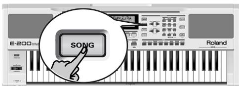
This is necessary because, otherwise, pressing the **START/STOP** button will start Arranger playback. So be sure to check whether the **SONG** button lights and whether the **ARRANGER** and **INTRO** **ORIGINAL** **FILL** **VARIATION** **ENDING** icons are no longer displayed. Only then will the **ARRANGER & SONG CONTROLS** buttons allow you to control song playback (see above).
