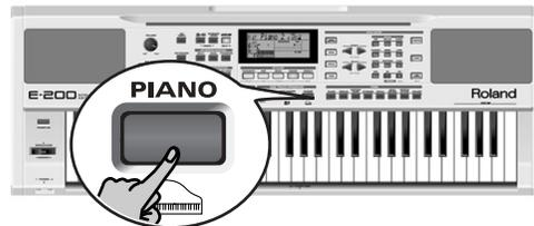
The **ARRANGER** icon disappears, the Arranger stops (if it was playing), and the E-200/E-100 automatically selects a piano sound for you.
