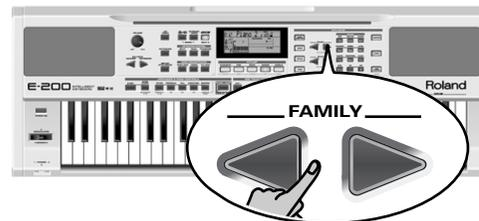
The E-200/E-100's Function parameters are divided into 9 logical "families". As the Bass Inversion parameter is an Arranger function, you need to select the Arranger settings (hence ARR SET).
