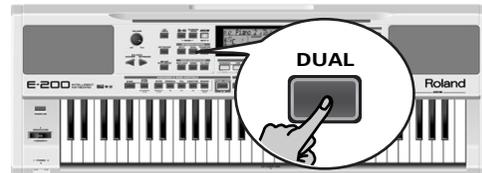
The **[DUAL]** icon appears and the E-200/E-100 now automatically selects a sound for the Dual part that complements the sound assigned to the Main part.
