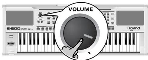
**Note:** When the E-200/E-100 is used at excessive volumes, the protection system of its power amplifier stage may come on and mute the speakers. In that case, reduce the volume setting and wait a few seconds.
