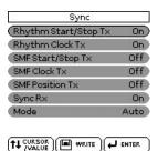
The "Sync" parameters allow you to specify whether or not the BK-5 should send MIDI real-time messages when you start rhythm or song playback. This allows you to synchronize external instruments or (software) sequencers with your BK-5.
