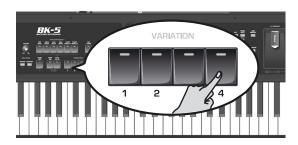
The VARIATION [4] button lights, while VARIATION [3] keeps flashing. The loop's start and end positions have been set and can be used.
