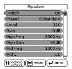
The equalizer has the same function as the TREBLE, MID and BASS knobs on a mixer: it allows you to color the sound, or to apply tonal corrections.
