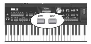
If you switch on one of these parts, the cursor on the main page automatically jumps to the "UP2" or "LWR" field. If [UP2] and [LWR] are both switched off, the cursor jumps to the "UP1" field.
