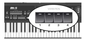
These buttons are used to select the complexity (number of parts) of the rhythm's arrangement:
