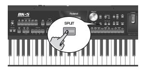
The BK-5 is now in Split mode: note numbers below the split point (see "Split" on p. 56) are used to transpose rhythm playback in real-time and to play the LWR part (if it is active). Note numbers above the split point can be used to play melodies using the UP1 and/or UP2 part.
