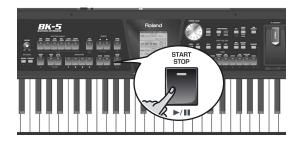
This button is used to start and stop rhythm playback. While a rhythm is running, the button's indicator flashes red on the first beat of each bar, and green on the remaining beats.
