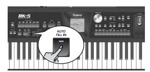
When this button lights, the BK-5 plays a transition before switching to the newly selected VARIATION pattern. Example: if the VARIATION [1] pattern is running, pressing the [4] button will not switch to that pattern right away—the BK-5 first plays a fill-in to announce the new song section.
