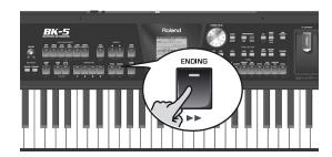
This button allows you to end your songs with a suitable closing section if you don't want to simply stop playback. The behavior of the Ending pattern depends on when you press the [ENDING] button:
