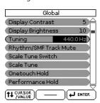
This parameter allows you to tune your BK-5 to acoustic instruments that cannot be tuned. The default is 440.0Hz.
