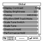
On this display page, "Display Contrast", "Display Brightness" and "Tuning" can be changed directly. The remaining entries provide access to additional display pages.
