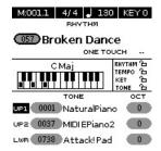
The display shows the current octave setting ("OCT") for all 3 real-time parts.
