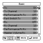
The Basic channel is used to receive and transmit Program Change and Bank Select messages for selecting Performances, as well as for the reception and transmission of other kinds of messages that are not directly related to a specific MIDI channel.
