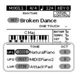
The highlighted numeric field refers to the part whose Tone assignment can be changed. To select a different part, move the cursor to its numeric field and press the [ENTER/SELECT] button.
