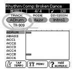
The field below the "TRACK" parameter shows the name of the Tone or Drum Set assigned to the selected track ("TR-909" in our example).
