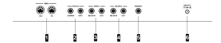
1. MIDI In/Out: These ports allow the instrument to be connected to other MIDI devices.
