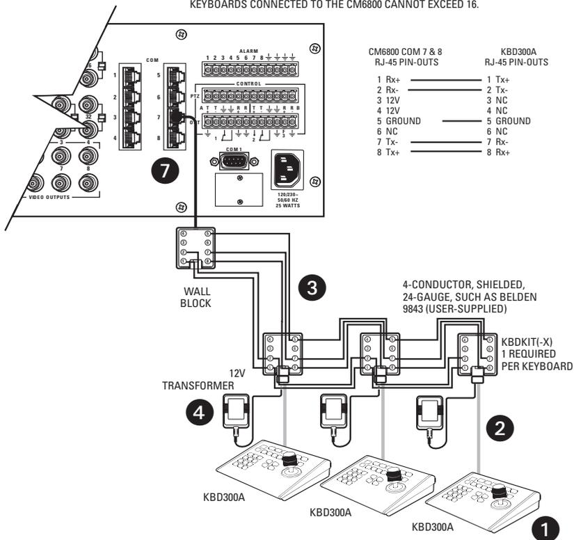
**Figure 4.** Connecting Remote Keyboards (CM6800-48X8 Shown)
