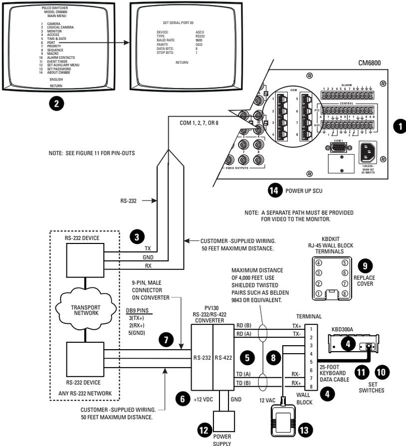
**Figure 7.** RS-232 Interface Connections (CM6800-48X8 Shown)
