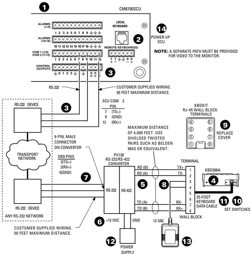
Figure 5. RS-232 Interface Connections (CM6700)
