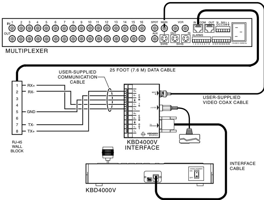
Figure 3. Connecting KBD4000V to a Multiplexer
