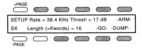
From this display, the DPM SX can be set up to "record" your favorite samples or sounds. As you can see from this menu, far more flexibility is available from the DPM 3SE control than is available from the front panel of the DPM SX. Since this allows for complete "remote" control of the DPM SX, it is not necessary to continually revisit your "rack gear" to reconfigure sampler parameters.
