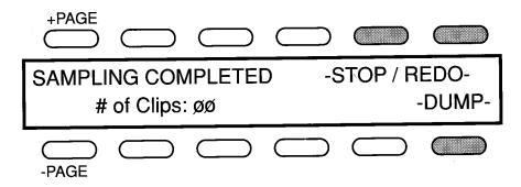
From this display, you can determine whether the sound sample suffered from any "clipping." The total number of times that the signal clipped is represented by the "# OF CLIPS: 00" display. This number should correspond to the number of times that the "clip" indicator flashed on the DPM SX. If you want to try again, simply depress the "STOP/REDO" soft button and the DPM 3SE will return to the DPM SX Setup menu.
