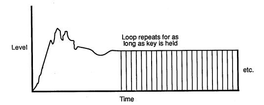
Since we no longer need the part of the sample that extends past the loop end, we can trim it off and reclaim a bunch of memory. Compare the figure below the original flute sample: The sample size has been cut in less than half, thus cutting memory requirements by more than half as well.
