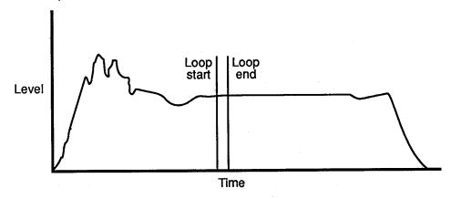
When you press a key, the sample plays normally until it reaches the end of the loop. It then jumps back to the loop start point and plays the looped section again, jumps back to the beginnings, plays through the loop again, and keeps repeating the looped section for as long as the key is held down. Thus, a looped sound can sustain indefinitely.
