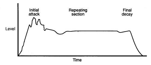
Note how there is a repeating section that occurs between the initial attack and final decay. This looks like a good place to create a loop; the following shows where we might put the loop.
