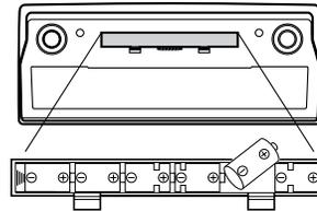
1. Press the tabs on the battery compartment cover, then pull up to remove the cover.
