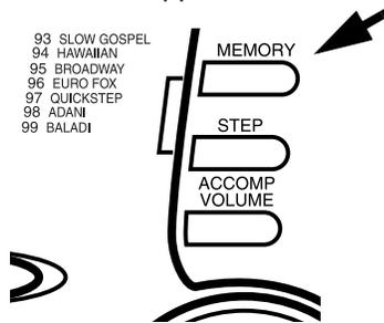
**Note:** **MEMORY** is a three-way switch. When you press it once, the keyboard enters the memory playback mode. When you press it again, it enters the memory record mode. When you press the button a third time, it turns off the memory function.
