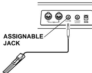
To connect a sustain pedal to your MD-1200, insert the plug on the pedal's cord into **ASSIGNABLE JACK** on the back of the keyboard.
