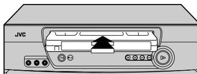
Make sure the window side is up, the rear label side is facing you and the arrow on the front of the cassette is pointing towards the VCR.
