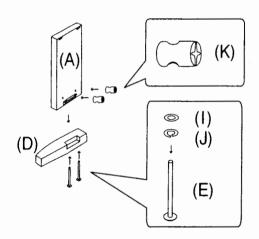
1. Insert the round nuts (K) into the holes of Side Panel (A) with keeping the nut's hole vertical. Insert the screws (E) into the spring washer and washer. Put (A) to Toe Block (D) and fasten with four screws (E) from the bottom.
