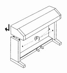
4. Place the piano on the stand. Then, slide the piano backward to place it at the appropriate point for screws. Hold the piano on the stand so that it doesn't fall from the stand. Then fasten the piano and the stand with four long screws.
