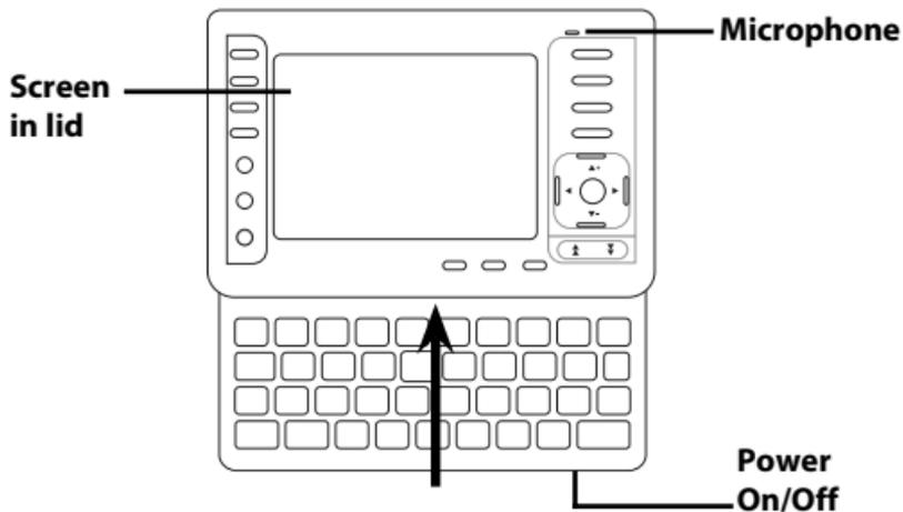
**Screen in lid:** The screen of your device is contained in the lid. To expose the keyboard, the lid must be moved up. Apply light pressure with your thumbs to the bottom of the device until you hear the lid move past the catch. Continue pushing the lid until you hear a snap, indicating that the lid can go no further.
