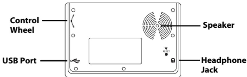
**Speaker:** The speaker is located in the upper right corner on the back of your device. For best results, do not cover the speaker.
