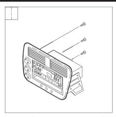
Mount the climate control pod to the back of the dash trim bezel with (3) Phillips screws previously removed in step #2.
