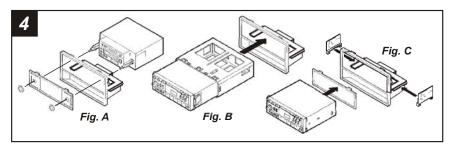
2-SHAFT HEAD UNITS: Snap the Faceplate into the Radio Housing. Slide the aftermarket head unit into the kit and secure with shaft nuts. (see Fig. A)
