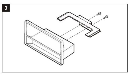
**ISO-DIN HEAD UNITS:** Mount the **Rear Support Bracket** to the back of the pocket with (2) **Phillips Screws** supplied. Skip to the Installation Instructions for ALL VEHICLES on Page #11.
