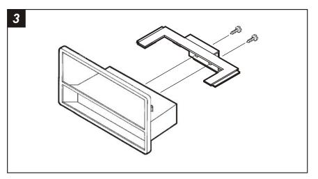
**ISO-DIN HEAD UNITS:** Mount the **Rear Support Bracket** to the back of the pocket with (2) **Phillips Screws** supplied. Skip to the Installation Instructions for ALL VEHICLES on Page #11.
