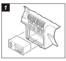
Disconnect the negative battery terminal to prevent an accidental short circuit. Remove (4) screws from the lower portion of the center console. Remove the gear shifter knob and lift the console out. Remove the ashtray and ashtray bracket. Remove (2) screws from the bottom of the head unit support, slide the unit out and disconnect the wiring.
