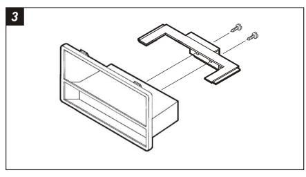
Mount the **Rear Support Bracket** to the back of the pocket with (2) **Phillips Screws** supplied. *Skip to the Installation Instructions for ALL VEHICLES on Page #11.*
