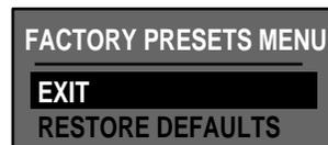
Press ▼ to highlight RESTORE DEFAULTS, then press SELECT. This will clear and reload all preset effects and all factory settings of Volume, Balance, Contrast, Configuration, etc. When the message FACTORY DEFAULTS RESTORED is displayed, press DONE to return to normal operation.
