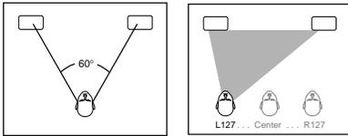
**SPEAKER ANGLE** is the angle between the main speakers as seen from the listening position — here it is about 60°. **LISTENER POS** allows you to adjust for an offset listening position.
