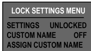
Locking the settings allows full operation of the unit but prohibits the ability to change effect parameters or setup values. Specifically, with the settings locked, the unit will allow any Parameter or Setup menu to be displayed, but attempting to select any item for adjustment will display the message: SETTINGS ARE LOCKED.
