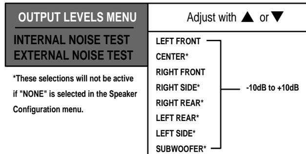
Using a Sound Pressure Level Meter such as Radio Shack model 33-2050 or 33-2055, set the weighting to *C* and the response to *Slow*. Adjust all output levels to achieve 75dB at the listening position.
