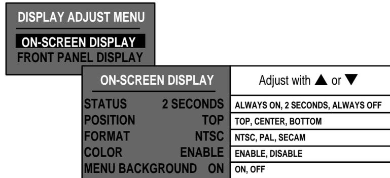
This menu allows you to choose the position and duration of items displayed on-screen during normal operation, as well as the options of color or black and white display and conformance to local video format.
