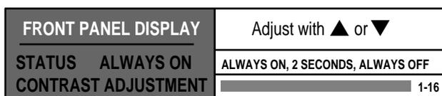
If you want to turn the front panel display off, use SELECT to highlight STATUS, then use ▲ or ▼ to select ALWAYS OFF. With software Version 4, you can select 2 SECONDS which will cause the display to shut off automatically two seconds after a command is received.
