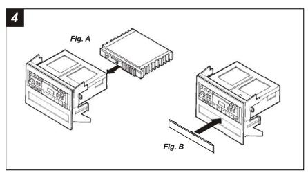
IF AN EQUALIZER WILL BE INCLUDED: Slide the aftermarket equalizer into the back of the Radio Housing. Using the hardware included with the equalizer, mount the unit to the kit. (see Fig. A)
