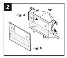
Cut and remove all mounting tabs on the *Radio Housing* EXCEPT tabs "B". The mounting tabs can be identified by the stamped letter on the back of each tab. (see Fig. A). Locate Faceplate #2. (see Fig. B). Skip to the Installation Instructions for ALL VEHICLES on Page #2.
