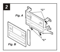
Cut and remove all mounting tabs on the *Radio Housing* EXCEPT tabs "C". The mounting tabs can be identified by the stamped letter on the back of each tab. (see Fig. A). Cut and remove the side portion of *Faceplate #1*. (see Fig. B). Skip to the Installation Instructions for ALL VEHICLES on Page #2.
