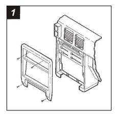
Disconnect the negative battery terminal to prevent an accidental short circuit. Remove the ashtray. Remove (2) screws from the base of the radio trim bezel. Remove (2) screws above the climate controls. Unclip the radio trim bezel and remove. Remove (4) screws securing the factory head unit and disconnect the wiring.
