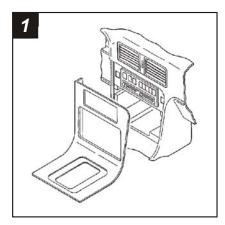
Disconnect the negative battery terminal to prevent an accidental short circuit. Unclip the gear shifter/radio trim bezel and remove the bezel. Remove (4) Phillips screws securing the factory head unit and disconnect the wiring.
