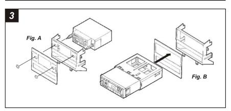
**2-SHAFT HEAD UNITS:** Attach the **Faceplate** to the **Radio Housing.** Slide the aftermarket head unit into the kit and secure with shaft nuts. (see Fig. A)
