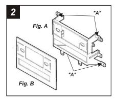
Cut and remove all mounting tabs on the *Radio Housing* EXCEPT tabs "A". The mounting tabs can be identified by the stamped letter on the back of each tab. (see Fig. A). Locate Faceplate #1. (see Fig. B). Skip to the Installation Instructions for ALL VEHICLES on Page #2.
