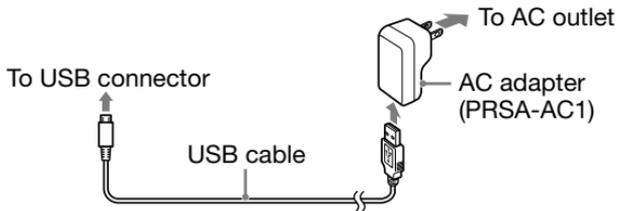
The Reader requires about 2 1/2 hours to fully charge (lights up red while charging), after which the charge/busy indicator goes off.
