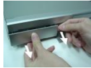
Step 3 Pull out the cartridge
