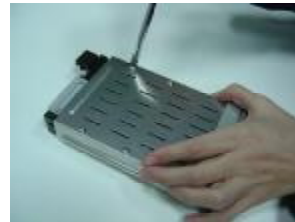
Step 4 Loose all screws on the Cartridge
