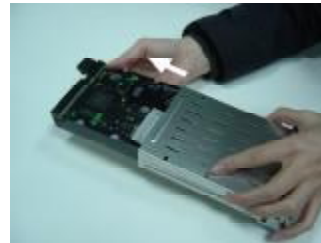
Step 5 Remove the HDD from Cartridge
