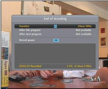
Pressing the  button will pause the live show and begin time shifting within the current recording even with the Time Shifting option disabled. However, it is still possible to pause a recording. After a recording is started, pressing the  button displays a menu like the left figure, in which you can set the recording duration.
