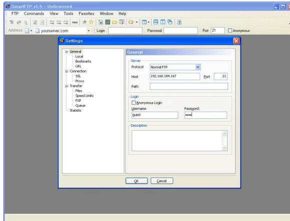
You can log into the FTP server with the user name and password specified in the WLAN Setting menu. For how to configure the WLAN settings, refer to § 8.2.
