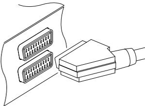
For best results with a standard television set, you should use a SCART cable. Plug one end of the cable into the TV socket on the digital receiver, and plug the other end into a free SCART socket on your television.
