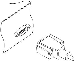
1. Plug one end of a RS-232 cable (9 pin D-sub cable) into the RS-232 port on the digital receiver, and the other end into the matching port on the other digital receiver.
