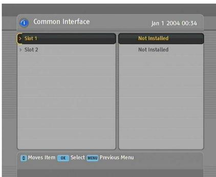
To view the information about the module and subscription card which is inserted into the digital receiver, select the Information > Common Interface menu. You should see a screen like the left figure.
