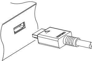
If you have a high definition television set, you should use a HDMI cable for best results. Plug one end of the cable into the HDMI socket on the digital receiver, and plug the other end into the matching socket on your television. In this case, you do not have to make audio connections because the HDMI connector can output stereo audio or Dolby digital audio.
