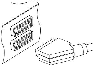
You will need to obtain a SCART cable to use the auxiliary SCART connector. Plug one end of the cable into the VCR socket on the digital receiver, and plug the other end into the matching socket on your video cassette recorder or suchlike.
