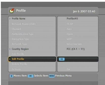
To make profiles for various network connections, select the Installation > LAN Setting > Profile menu.
