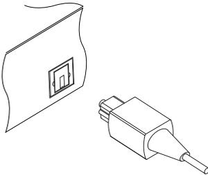
To enjoy Dolby digital audio, your television or audio system must be able to decode Dolby digital audio, and you will need to obtain a S/PDIF cable. Plug one end of the cable into the S/PDIF socket on the digital receiver, and plug the other end into the matching socket on your audio system.
