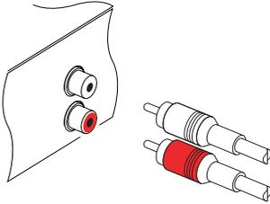
You will need to obtain an audio cable (RCA cable) to connect the audio connectors. Plug one end of the cable into the AUDIO L (white) and AUDIO R (red) sockets on the digital receiver, and plug the other end into the matching sockets on your television or audio system.
