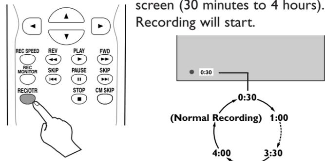
When the unit reaches the specified time, recording will stop automatically.
