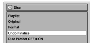
To release the finalizing for the disc, select “Undo Finalize” at step 3.
