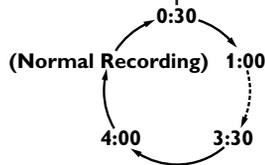
When the unit reaches the specified time, it will be turned off automatically.
