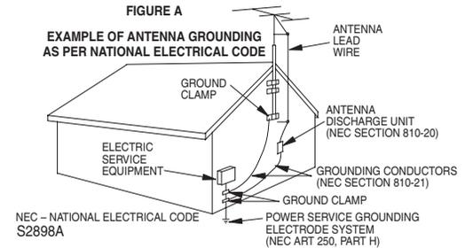
14. Lightning - For added protection for this product during a lightning storm, or when it is left unattended and unused for long periods of time, unplug it from the wall outlet and disconnect the antenna or cable system. This will prevent damage to the product due to lightning and power-line surges.
