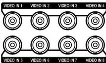
Connect the coaxial cables from the video sources to the BNC Video In connectors.
