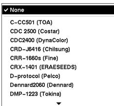
Highlight the box in the Product column for the PTZ camera you wish to configure and press the button. A list of PTZ devices appears. Select your camera from the list and press the button. You will need to connect the camera to the RS232 or RS485 connector on the back of the DVR following the camera manufacturer's instructions.
