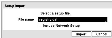
You can import saved DVR settings or export the current DVR settings. To import saved DVR settings, connect the USB device containing the setup file (.dat) to the DVR. Highlight **Setup – Import...** and press the
