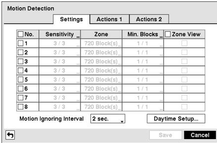
Figure 30 – Motion Detection Settings setup screen.
