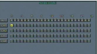
Schedule record can be set 24 hours per day. Press  $\checkmark \checkmark \checkmark \land$  move to the right time zone and select the desired record mode by using the ENT button.
