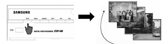
Press the AUTO button, and the Auto Screen Display Switching is released.
