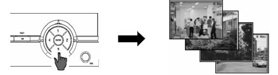
Press the ENT button, then the four connected channels are displayed on the quad split screens.
