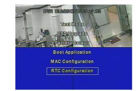
③ Move the cursor to RTC Configuration and press ENT button. Following screen appears.
