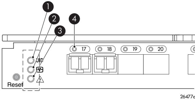
**Figure 6 Verifying power-on LEDs**
