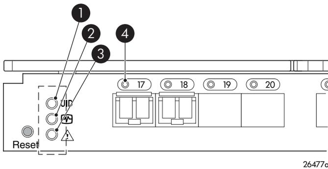
**Figure 8 Identifying LEDs**
