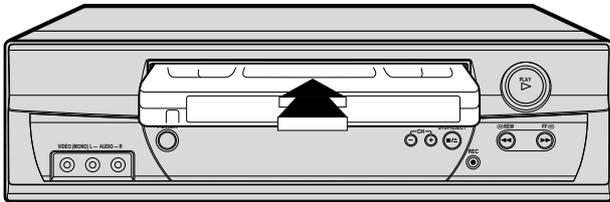
Make sure the window side is up, the rear label side is facing you and the arrow on the front of the cassette is pointing towards the VCR.
