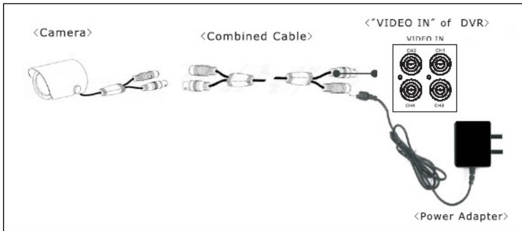
**<Connection Type2-For cameras that have a video output port on the rear>**
