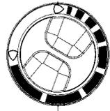
**B** As shown, you are able to regulate the temperature of the cooling compartment, if necessary, by turning rotary knob (B) .
