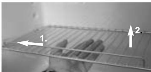
2. Move the storage rack to the left and remove it.
