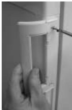
2. Adjust door handle at the door and screw onto it.
