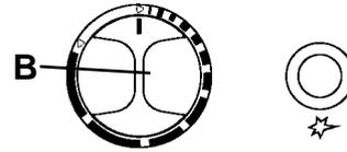
2. Use rotary switch (B) to regulate the temperature in the main refrigerator compartment.
