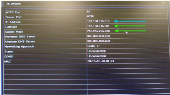
Then return to the Network setup screen and enter this information into the table in the configuration screen (shown below) and remove checkmark from the Obtain IP address box Next click on the Apply button to save the addresses So the router does not change them.
