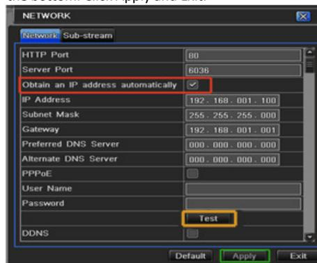
After the router has assigned the DVR an IP address Go back to the Main Menu and click on the Information Icon then Network Icon and write down the IP address, Subnet Mask, and Gateway assigned by the router
