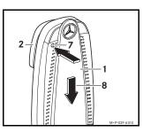
Press and hold the release button (7). Slide the Mercedes-Benz Cradle adaptor with Bluetooth® (1) in direction of arrow (8) and remove it from the pre-installed contact plate (2).
