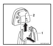
Insert the Mercedes-Benz Cradle adaptor with Bluetooth  $^{\otimes}$  (1) into the latches on the pre-installed contact plate (2), located in the center console. To insert the Mercedes-Benz Cradle adaptor with Bluetooth® (1), slide it upwards until it clicks into place.
