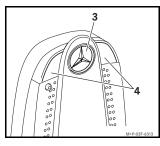
With Mercedes-Benz Cradle adaptor with Bluetooth® connected to the vehicle press button (3) for approx. 2-3 seconds.
