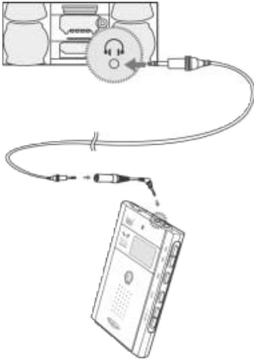
① Connect the audio cable to micro- phone jack of the RipFlash Trio using the earphone connector(a) and connect the other head of audio cable to the earphone jack of the audio devices.
