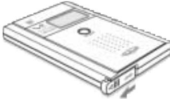
① Slide the battery cover in the direction of the arrow.
