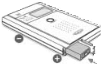
③ Insert the rechargeable battery as shown in the picture. Adjust the (+)(-) polarities of the batteries in the compartment.
