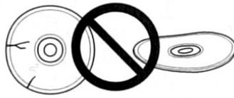
Non-standard disc shapes are unusable on this drive. These non-standard shapes include hearts, diamonds, polygons, etc.
