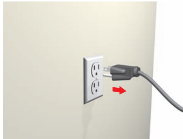
Figure 3. Removing Power Cord from Wall
