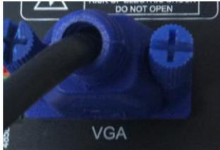
2. Connect the other end of the cable to an available VGA input on your TV or monitor.
