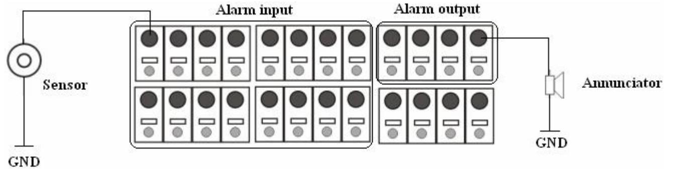
**Attention:** The alarm output is TTL high level control. The connection method is described in detail in the Above picture.
