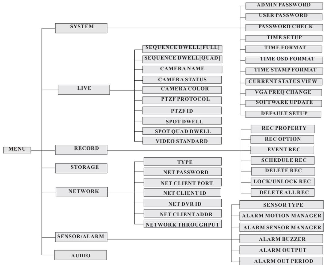
There are two users in the origin DVR system. One is Admin which has highest priority to set system's configuration and whose password is "0000", the other is common user which is just allowed to see the live play and the playback picture and does not have the right to change the user password, which is done by Admin users.
