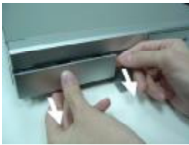
Step 3 Pull out the cartridge
