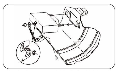
Using a perforated support strap, mount the back of the unit tosub-dash. the rear support location in the sub-dash.
