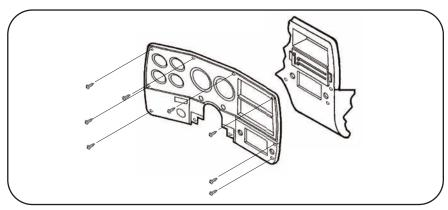
**SHAFT HEAD UNITS:** Position the Faceplate against the face of the radio trim bezel and slide it to the right until the right edge of the Faceplate meets the lip of the bezel. (see Fig. A). Slide the aftermarket head unit through the sub-dash, dash trim bezel and Faceplate and secure with shaft nuts. (see Fig. B). Skip to Final assembly.
