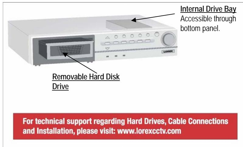
The internal drive bay is located in the bottom panel of the DVR as referenced above.
