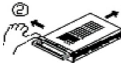
3. **Connect the HDD into the Cartridge Casing**
