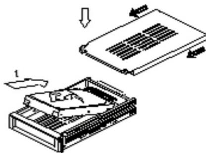
6. **Reinsert the Cartridge Casing into the DVR**
