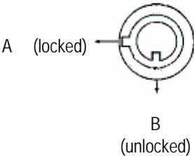
If you need to unlock the cabinet, turn the key counter-clockwise from the position shown above.
