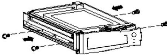
5. **Slide the top Cover over the Cartridge Casing**
