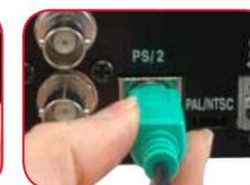
PS/2 - (Optional Connection) - PS/2 port to connect a serial Mouse to the DVR unit. Used for mouse navigation of the menus.
