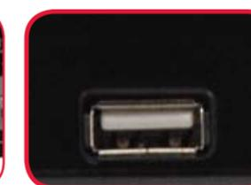
USB PORT - Provides connection port for USB Flash Drives (thumbsticks).
