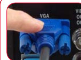
VGA VIDEO OUTPUT (Optional Connection) - Video Output port to connect the unit to a Computer Monitor.
