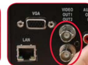
BNC VIDEO OUT - Video Output port to connect the unit to another recording device or monitor
