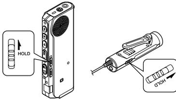
**Setting the HOLD switch to the HOLD position.** If you set the recorder to HOLD status by sliding the HOLD switch in the direction of the arrow, the current conditions will be preserved, and all buttons and switches except the HOLD switch will be disabled. This feature is useful when the recorder has to be carried in a bag or pocket. **Remember to reset the HOLD switch when using the recorder.**
