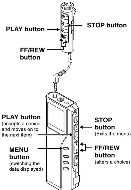
When the remote controller microphone is connected, buttons with the same names as those on the recorder work analogously.
