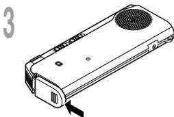
1 Lightly press down on the arrow and slide the battery cover open.
